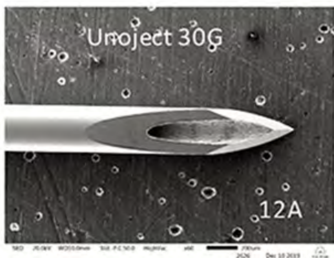
Figura 3: Bisel trifacetado da Unoject 30G. Fonte: Monteiro MAO, Antunes ANDG, Basting RT. Physical, chemical, mechanical, and micromorphological characterization of dental needles. J Dent Anesth Pain Med. 2021 Apr;21(2):139-153.
